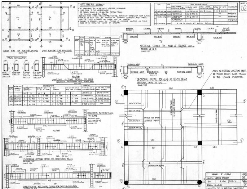
Figure 9b: Graphical Expression of design and construction R.C.C slab and beams (Image Source: Authors).
